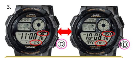
Press (D) button to toggle between Daylight Saving Time (on) and Standard Time (off).
