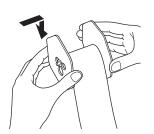
**6** Place the take-up reel into place behind the printer, above the roll paper.
