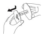
**4** Slide the leading end of the paper into the groove on the spindle of the take-up reel and wind it onto the reel two or three turns.
