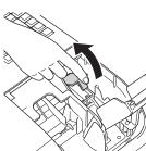
3 Note the (+) and (-) markings in the battery compartment. Load a set of two new "AA" type manganese batteries so that their plus (+) and minus (-) ends are facing as indicated by the markings.
