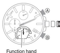
9. If the function hand and/or the day indicator is out of alignment, rotate the crown to adjust them. Move the function hand to 12 o'clock and/or the day to the center of the indicator window.
