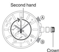
3. Rotate the crown to align the second hand with 12 o'clock.
