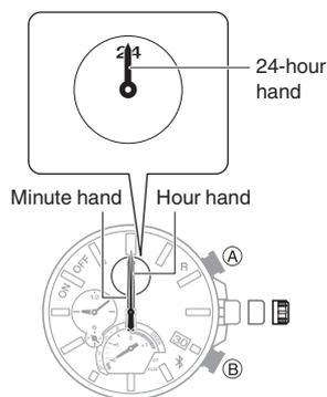
5. Rotate the crown to align the hour hand, minute hand, and 24-hour hand with 12 o'clock.
