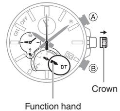
2. Rotate the crown to change the Dual Time setting.
