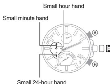
7. Rotate the crown to align the small hour hand, small minute hand, and small 24-hour hand with 12 o'clock.
