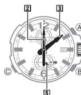
1. In the Timekeeping Mode, press **(C)** three times to enter the Countdown Timer Mode.
