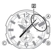
In the Timekeeping Mode, press **B**. The **[2] Second Hand** will move to **Y (YES)** or **N (NO)** to indicate the last calibration signal receive result.
