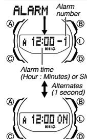
You can set five independent daily alarms. When a daily alarm is turned on, an alarm tone will sound for about 10 seconds each day when the time in the Timekeeping Mode reaches the preset alarm time. This is true even if the watch is not in the Timekeeping Mode. You can also turn on an Hourly Time Signal, which will cause the watch to beep twice every hour on the hour.
