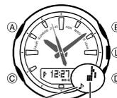
Current alarm on indicator (currently display alarm on)
