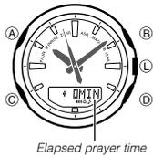
While the Today's Salat Time Screen is displayed, the digital display will show the time elapsed for up to 30 minutes after the start of the prayer. The second hand will remain pointing to the name of the ongoing prayer. Elapsed prayer time is shown only while Today's Salat Time Screen is displayed.
