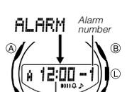
You can set five independent daily alarms. When a daily alarm is turned on, an alarm tone will sound for about 10 seconds each day when the time in the Timekeeping Mode reaches the preset alarm time. This is true even if the watch is not in the Timekeeping Mode. You can also turn on an Hourly Time Signal, which will cause the watch to beep twice every hour on the hour.
