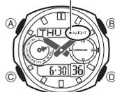
An LED (light-emitting diode) illuminates the face of the watch for easy reading in the dark. The watch's auto light switch turns on illumination automatically when you angle the watch towards your face.
