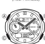
When an alarm is turned on, the alarm tone will sound when its alarm time is reached. One of the alarms is a snooze alarm, while the other four are one-time alarms.
