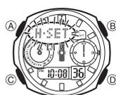
In the Timekeeping Mode, hold down **(D)** for about six seconds, until **H-SET** starts flashing on the upper display.
