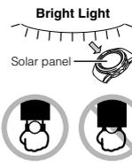
The electricity generated by the solar panel of the watch is stored by a built-in battery. Leaving or using the watch where it is not exposed to light causes the battery to run down. Make sure the watch is exposed to light as much as possible.
