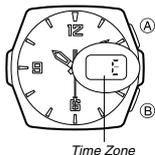
1. In the Timekeeping Mode, hold down (B) for about five seconds until the currently selected Time Zone appears on the display. This is the setting mode.
