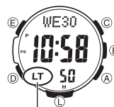
Auto light switch on indicator
