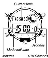
The countdown alarm can be set within a range of 1 second to 24 hours. When the countdown reaches zero, an alarm sounds for 10 seconds or until you press any button.
