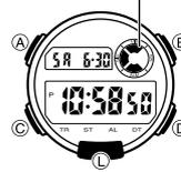
In the Timekeeping Mode, hold down (D) for about two seconds to toggle the Vibration Alarm between on (Vibration Alarm on indicator displayed) and off (indicator not displayed).
