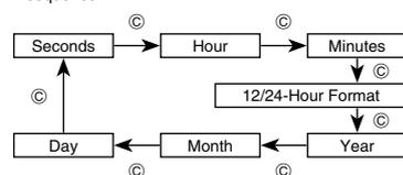
3. While the seconds digits are selected (flashing), press **(D)** to reset the seconds to 00. If you press **(D)** while the seconds count is in the range of 30 to 59, the seconds are reset to 00 and 1 is added to the minutes. If the seconds count is in the range of 00 to 29, the minutes count is unchanged.
