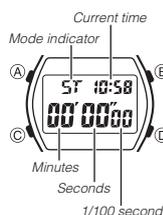
The stopwatch lets you measure elapsed time, split times, and two finishes. The range of the stopwatch is 23 hours, 59 minutes, 59 seconds.
