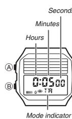
The countdown timer can be set within a range of one minute to 24 hours. An alarm sounds when the countdown reaches zero.
