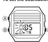
1. In the Countdown Timer Mode, press (A) until the hours of the countdown start time start to flash. This is the setting screen.
