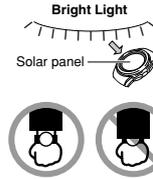
The electricity generated by the solar panel of the watch is stored by a rechargeable battery. Leaving the watch where it is not exposed to light causes the battery to run down. Make sure the watch is exposed to light as much as possible.
