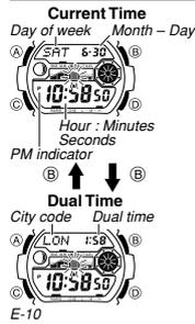
Press the (B) button to toggle the upper display between the day of the week and date, and the currently selected World Time city and time (Dual Time). Use the Timekeeping Mode to set and view the current time and date.
