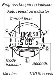
The countdown alarm can be set within a range of 1 second to 24 hours. When the countdown reaches zero, an alarm sounds for 10 seconds or until you press any button.
