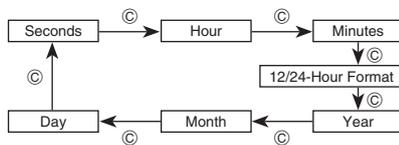
3. While the seconds digits are selected (flashing), press **(D)** to reset the seconds to 00. If you press **(D)** while the seconds count is in the range of 30 to 59, the seconds are reset to 00 and 1 is added to the minutes. If the seconds count is in the range of 00 to 29, the minutes count is unchanged.
