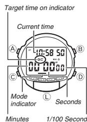
The Stopwatch Mode lets you measure elapsed time, split times, and two finishes. The range of the stopwatch is 23 hour, 59 minutes, 59.99 seconds. You can also have an alarm sound when a target time is reached. The Stopwatch Mode also features an Auto-Start function.
