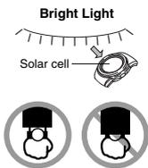
The electricity generated by the solar cell of the watch is stored by a built-in battery. Leaving or using the watch where it is not exposed to light causes the battery to run down. Make sure the watch is exposed to light as much as possible.
