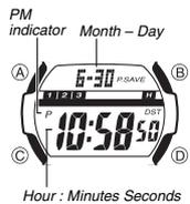
This watch receives a time calibration signal and updates its time setting accordingly. The time calibration signal includes both Standard Time and Daylight Saving Time (summer time) data.
