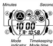
The countdown timer can be set within a range of one minute to 60 minutes. An alarm sounds when the countdown reaches zero. The countdown timer has two modes: auto-repeat and elapsed time, and a progress beeper signals the progress of the countdown. All of this makes the countdown timer a valuable tool for timing the start of a yacht race.
