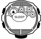
If the **SLEEP** indicator is on the display, it means that the display is blank because the watch's Power Saving function has turned off the display to conserve power. Power Saving automatically turns off the display and enters a sleep state whenever your watch is left for a certain period where it is dark.
