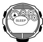
When turned on, the Power Saving function automatically puts the watch into a sleep state whenever it is left in an area where it is dark for 30 to 35 minutes. The sleep state is indicated by a blank screen with **SLEEP** flashing on it. In the sleep state, all functions are enabled, except for the display.
