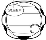
If the sleep indicator (SLEEP) is displayed, it means the watch's Power Saving function has turned off the display to conserve power. Power Saving automatically turns off the display and enters a sleep state whenever the watch is left for a certain period where it is dark.
