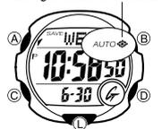
The backlight uses an EL (electro-luminescent) panel that causes the entire display to glow for easy reading in the dark. The watch's auto light switch automatically turns on the backlight when you angle the watch towards your face in the dark.
