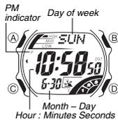
This watch receives a time calibration signal and updates its time setting accordingly. The time calibration signal includes both Standard Time and Daylight Saving Time (summer time) data.
