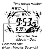
The Time Recorder lets you store up to 30 records of the current time (month, day, hour, minutes, seconds, and DST on/off setting) with the touch of a button. One way you can use the Time Recorder is to record the start time and the end time of a particular event.
