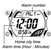
The Alarm Mode gives you a choice of four one-time alarms and one snooze alarm. Also use the Alarm Mode to turn the Hourly Time Signal (SIG) on and off.
