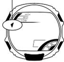
If the sleep indicator (S4/SLEEP4) is on the display, it means that the display is blank because the watch's Power Saving function has shut it off to conserve power. Power Saving automatically turns off the display and enters a sleep state whenever your watch is left in an area where it is dark for a certain period.
