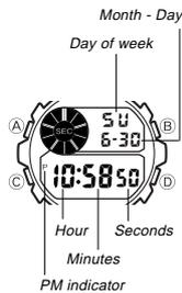
3. While the seconds digits are selected (flashing), press **D** to reset the seconds to "00". If you press **D** while the seconds count is in the range of 30 to 59, the seconds are reset to "00" and 1 is added to the minutes. If the seconds count is in the range of 00 to 29, the minutes count is unchanged.
