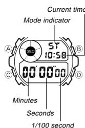
The Stopwatch Mode lets you measure elapsed time, split times, and two finishes. The range of the stopwatch is 23 hours, 59 minutes, 59.99 seconds.
