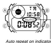
1. Press **(A)** while in the Countdown Alarm Mode. The hours digit flashes on the display because it is *selected*.
