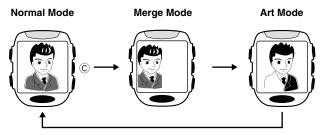
The recording mode you select remains in effect until you change it or exit the Camera Mode. The Normal Mode is the initial default whenever you enter the Camera Mode.
