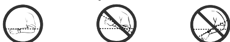
Parallel to ground More than 15 degrees too high More than 15 degrees too low
