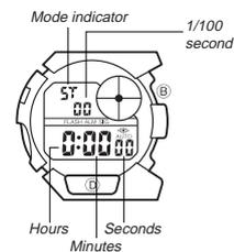
The stopwatch Mode lets you measure elapsed time, split times, and two finishes. The range of the stopwatch is 23 hours, 59 minutes, 59.99 seconds. You can use the EL backlight at any time while the stopwatch is operating.
