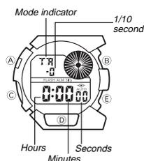
The countdown alarm can be set within a range of 1 second to 24 hours. When the countdown reaches zero, an alarm sounds for 10 seconds or until you press any button.
