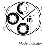
When the time shown on the display does not match the analog setting, use this mode to correct the analog setting.
