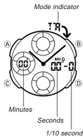
The countdown timer can be set within a range of 1 second to 60 minutes. When the countdown reaches zero, an alarm sounds for 10 seconds or until you press any button.
