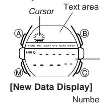
1. In the Telememo Mode, press (B) and (C) at the same time to display the new data display.
