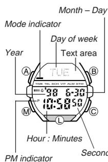
In addition to normal timekeeping, the Timekeeping Mode is also used to set the current time and date. You can also adjust the seconds count to "00" at any time by pressing two buttons.
