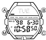
The Auto Display function continually changes the contents of the text area of the display. Note that you cannot use any of the watch's other functions (except for turning on the backlight) while the Auto Display function is operating.
