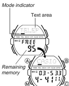
The Telememo Mode lets you store up to 100\* pairs of name and telephone number data. Stored data is sorted automatically into alphabetic sequence based on the text area text.
