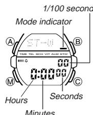
The Stopwatch Mode lets you measure elapsed time, split times, and two finishes. The range of the stopwatch is 23 hours, 59 minutes, 59.99 seconds.
