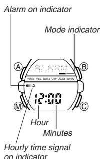
When the Daily Alarm is switched on, the alarm sounds for 20 seconds at the preset time each day. Press any button to stop the alarm after it starts to sound.
