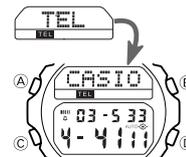
The Telememo Mode lets you store up to 30 pairs of name and telephone number data. The name can be up to 8 characters long and the number up to 12 digits. Data is automatically sorted into alphabetical order based on the name data. You can recall data by scrolling through it on the display.
