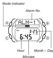
You can set five independent alarms with the hour, minutes, month and day. Use the Alarm Mode to turn the alarm and the Hourly Time Signal on and off.
