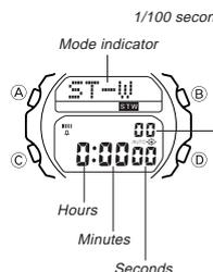
The Stopwatch Mode lets you measure elapsed time, split times, and two finishes. The range of the stopwatch is 23 hours, 59 minutes, 59.99 seconds.
