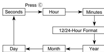
3. While the seconds digits are selected (flashing), press **B** to reset the seconds to "00". If you press **B** while the seconds count is in the range of 30 to 59, it is reset to "00" and 1 is added to the minutes. If the seconds count is in the range of 00 to 29, the minutes count is unchanged.
