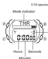
The countdown timer can be set within a range of 1 second to 24 hours. When the countdown reaches zero, an alarm sounds for 10 seconds or until you press any button.
