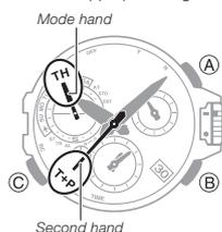
2. Hold down (B) for at least three seconds until the second hand moves to **T+P**. If the second hand moves to any other position besides **T+P**, keep (B) depressed until it moves to **T+P**.
