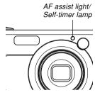
You can interrupt an ongoing self-timer countdown by pressing the shutter button while the AF assist light/self-timer lamp is flashing.
