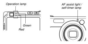
\* There are three lamp flash patterns. Pattern 1 flashes once per second, Pattern 2 flashes twice per second, and Pattern 3 flashes four times per second. The table below explains what each flash pattern indicates.
