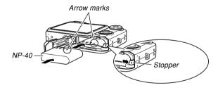
• Push the bottom of the battery, and make sure that the stopper securely locks the battery in place.
