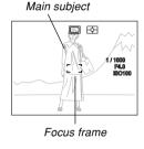
2. Keeping the shutter button pressed half way down, recompose the image as vou like.
