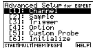
4. If you want to configure a custom probe at this point, press **[5]** (Custom Probe). Next, follow the steps under “To configure a custom probe starting from the Advanced Setup menu” on page 2-12.
