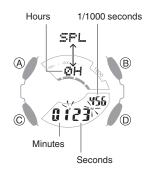
4. Press (A) to reset the measurement time to all zeros.
