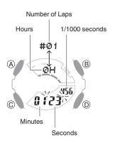
4. Press (A) to reset the measurement time to all zeros.
