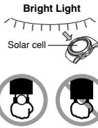
The electricity generated by the solar cell of the watch is stored by a built-in battery. Leaving or using the watch where it is not exposed to light causes the battery to run down. Make sure the watch is exposed to light as much as possible.
