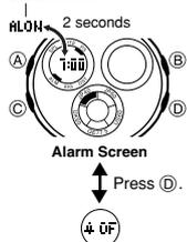
When the alarm is turned on, the alarm sounds when the alarm time is reached. You can also turn on an Hourly Time Signal, which will cause the watch to beep twice every hour on the hour.
