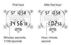
3. Press (B) to reset the measurement time to all zeros.
