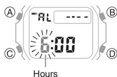
3. Keep pressing (C) until the setting you want to change is flashing.
