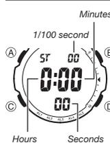
The stopwatch lets you measure elapsed time, split times, and two finishes.
