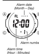
You can set up to five independent multi-function alarms with hour, minutes, month, and day. When an alarm is turned on, the alarm tone sounds when the alarm time is reached. One of the alarms has a snooze feature.
