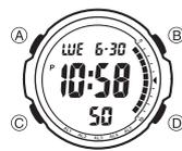
The backlight uses an LED (light-emitting diode) and a light guide panel that cause the entire display to glow for easy reading in the dark.
