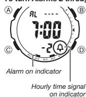
1. In the Alarm Mode, use (D) to select alarm number 2 through 5, or the Hourly Time Signal (:00).
