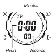
The countdown timer can be set within a range of one minute to 24 hours. An alarm sounds when the countdown reaches zero.
