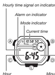
When the Daily Alarm is switched on, the alarm sounds for 20 seconds at the preset time each day. Press any button to stop the alarm after it starts to sound. When the Hourly Time Signal is on, the watch beeps every hour on the hour.
