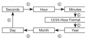
3. While the seconds digits are selected (flashing), press (D) to reset the seconds to 00. If you press (D) while the seconds count is in the range of 30 to 59, the seconds are reset to 00 and 1 is added to the minutes. If the seconds count is in the range of 00 to 29, the minutes count is unchanged.
