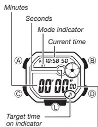
The Stopwatch Mode lets you measure elapsed time, split times, and two finishes. The range of the stopwatch is 23 hour, 59 minutes, 59.99 seconds. You can also have an alarm sound when a target time is reached. The Stopwatch Mode also features an Auto-Start function.
