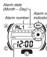
This watch has five independent multi-function alarms (including one snooze alarm). When an alarm is turned on, the alarm tone sounds when the alarm time is reached. You also can turn on an Hourly Time Signal that causes the watch to beep twice every hour on the hour.
