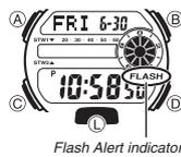
When Flash Alert is turned on, the illumination flashes for the alarms, the Hourly Time Signal, the countdown alarm, and stopwatch (ST1) auto start.
