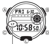
This watch has an EL (electro-luminescent) panel that causes the entire display to glow for easy reading in the dark. The auto light turns on illumination automatically when you angle the watch towards your face for reading.
