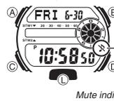
The button operation tone sounds any time you press one of the watch's buttons. You can turn the button operation tone on or off as desired.
