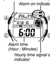
After you set (and turn on) the daily alarm, the alarm tone sounds when the alarm time is reached. You can also turn on an Hourly Time Signal that causes the watch to beep for about one second every hour on the hour.
