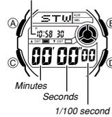
The stopwatch lets you measure elapsed time, split times, and two finishes.
