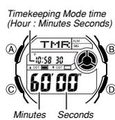
You can set the countdown timer within a range of one to 60 minutes. An alarm sounds when the countdown reaches zero.
