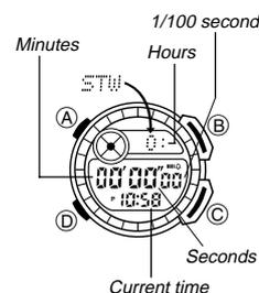
The Stopwatch Mode lets you measure elapsed time, split times, and two finishes. The range of the stopwatch is 23 hours, 59 minutes, 59.99 seconds.
