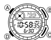
1. In the Timekeeping Mode, hold down (A) until the seconds digits start to flash on the display.
