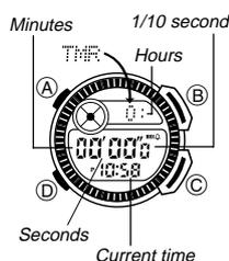
The countdown timer can be set within a range of 1 second to 24 hours. When the countdown reaches zero, an alarm sounds.
