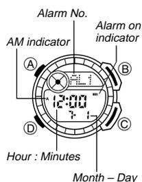
You can use the Alarm Mode to set three independent alarms with hour, minutes, month, and day. You can also turn on an Hourly Time Signal that causes the watch to beep twice every hour on the hour.
