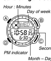
Use the following procedure to calibrate the seconds count on a time signal from a radio, TV, or other source.
