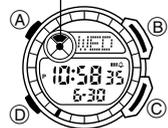
The backlight uses an EL (electro-luminescent) panel that causes the entire display to glow for easy reading in the dark. The watch's auto light switch automatically turns on the backlight when you angle the watch towards your face.
