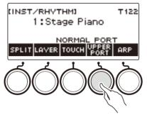
• If the SUS button is displayed, switch it to the UPPER PORT button (page EN-84).
