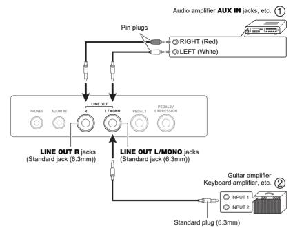
• When connected with an audio device (Figure ①) LINE OUT R (right) is the right channel and LINE OUT L/MONO (left) is the left channel. Use a commercially available connection cable for connection as shown in Figure ①. Normally, you should set the input selector of the audio equipment to the jack where the Digital Keyboard is connected (AUX IN, etc.)
