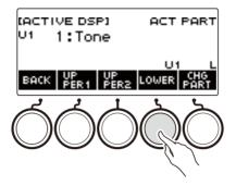
**6** Press UPPER1, UPPER2, or LOWER to select the part for which you want to disable application of the effect. This causes the selected part indicator ("U1", "U2", "L") to disappear from the lower right of the display.
