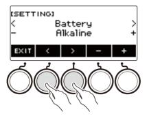
6. Rotate the dial or use – and + to select "Alkaline" (alkaline batteries) or "Ni-MH" (nickel-metal hydride batteries).
