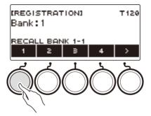
• If the last recalled bank number is selected, the area number will be displayed at the bottom of the LCD.
