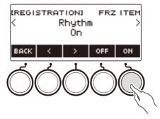
• If an item's status is currently FRZ ITEM ON (not recalled), you can change it back to FRZ ITEM OFF (recalled) by rotating the dial to the left or by pressing OFF. This displays "Off" for the setting.
