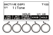
5. Press HOLD again to return to the DSP screen and turn off Active DSP.
