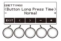
**5.** Rotate the dial or use – and + to change the button long-press time value.
