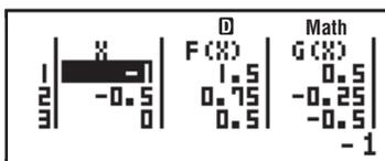
**Note:** • The maximum number of rows in the generated number table depends on the setup menu table setting. Up to 30 rows are supported for the “f(x)” setting, while 20 rows are supported for the “f(x),g(x)” setting. • You can use the number table screen for viewing values only. Table contents cannot be edited. • The number table generation operation causes the contents of variable X to be changed.
