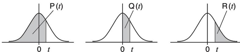
**▶t:** This function is preceded by the argument X, and determines the normalized variate  $X \blacktriangleright t = \frac{X - \bar{x}}{\sigma_x}$ .
