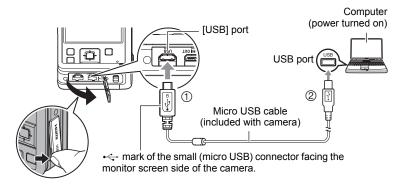
If the camera is on, press [ON/OFF] (Power) to turn it off before connecting it to your computer.
