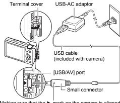
Making sure that the ▶ mark on the camera is aligned with the ◀ mark of the USB cable connector, connect the cable to the camera.
