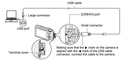
The camera will turn on automatically and battery charging will start (page 19).
