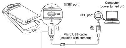
• mark of the small (micro USB) connector facing the side opposite that of the monitor screen.
