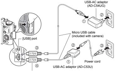
• crimer mark of the small (micro USB) connector facing the monitor screen side of the camera.
