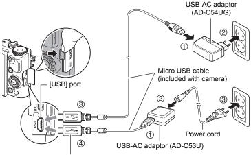
• mark of the small (micro USB) connector facing the monitor screen side of the camera.
