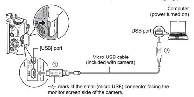
If the camera is on, press [ON/OFF] (Power) to turn it off before connecting it to your computer.
