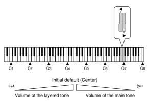
To return the volume setting to its initial default, hold down the FUNCTION button and press both of the keys at the same time.
