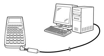
After you finish data communications, turn off power in the sequence: the unit first, and then the personal computer. Finally, disconnect the equipment.
