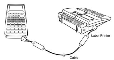
After you finish data communications, turn off power in the sequence: the unit first, and then the Label Printer. Finally, disconnect the equipment.
