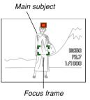
Keeping the shutter button pressed half way down, recompose the image as you like.
