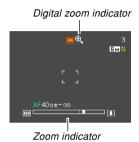
2. When the zoom pointer reaches the optical/digital zoom switch over point, it will stop.
