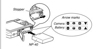
• Push the bottom of the battery, and make sure that the stopper securely locks the battery in place.
