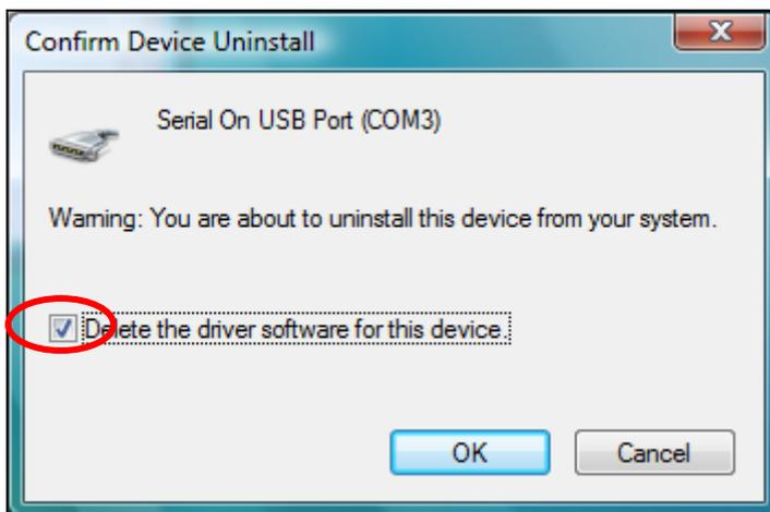
5) Disconnect the SB-88 cable from the computer, and then reconnect it. Now install the correct driver using the procedure under "Installing the SB-88 Cable Driver".
